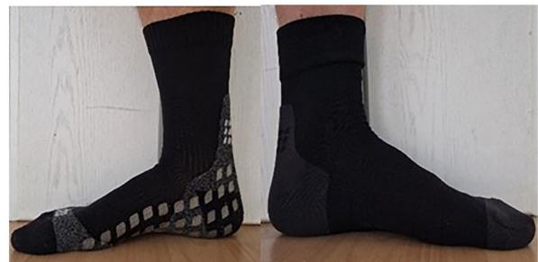
Figure 1. Experimental socks; GripSock (left) with frictional enhancing dots, CompressionS (right).
